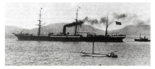
**S.S. Kaikoura -** New Zealand Shipping Co. 1884-1899 Built: 1884 by John Elder & Co., Glasgow Tonnage: 4,474/gross/2,780 net Dimensions: 430 x 46 ft/131.1 x 14 m.
